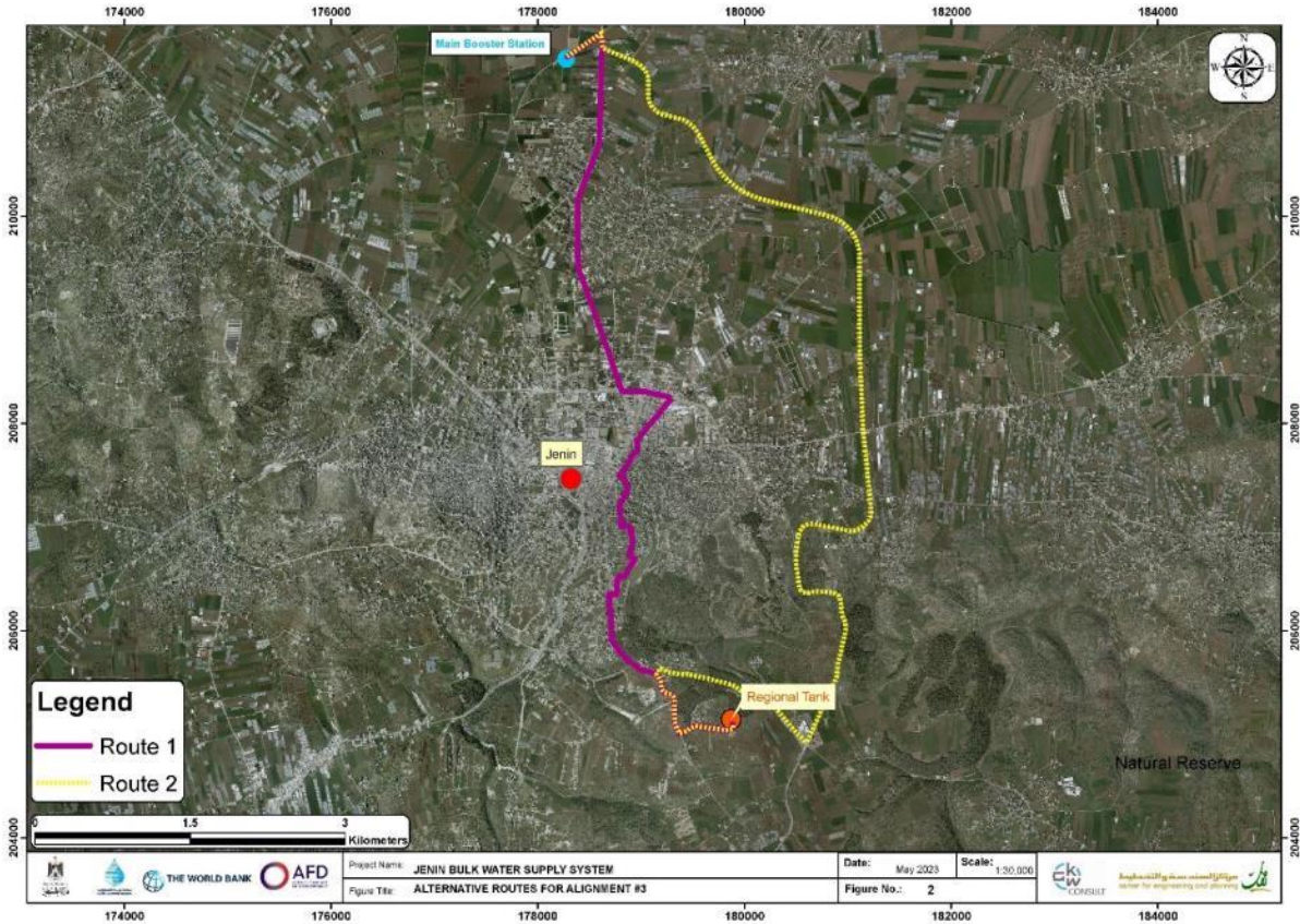
Figure 2-9: Alternative Routes for Alignment #3 from Main Booster Station to Regional Tank (Source: Consultant)
